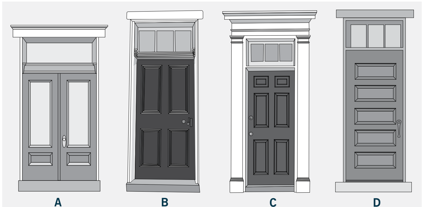
5-17 (A–D) Paneled doors installed on residences in the Historic District are evident in a number of configurations. The four- and six- panel doors are the most common doors on Frederick's early houses, and the five-panel door usually indicates twentieth century construction or a replacement door.
