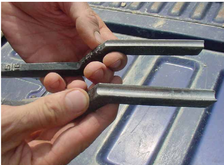
4-16 Masons use special tools to repoint brick with historical accuracy. These tools are used to make beaded mortar joints.
