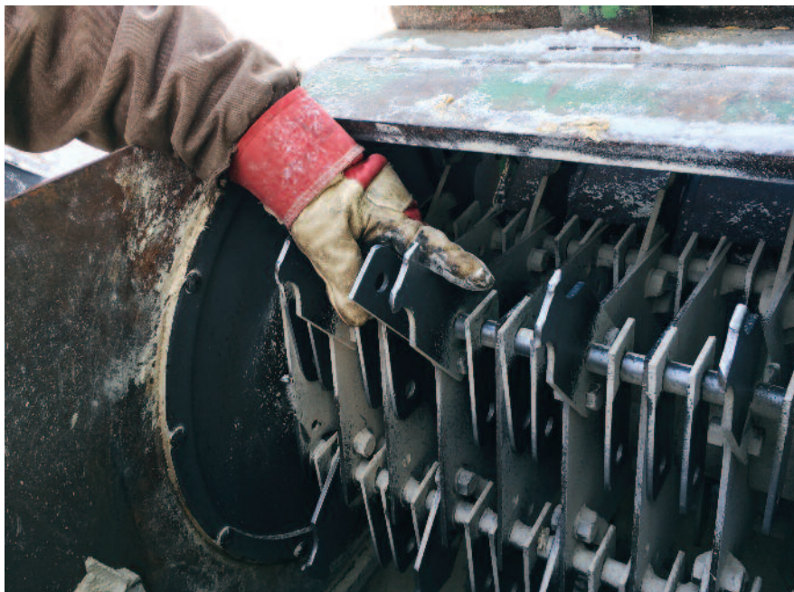
Checking hammer-mill flails for wear and proper function helps ensure feed is processed accurately.
