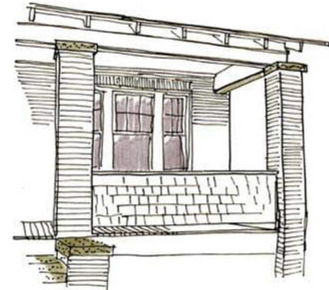
Brick Pier with Concrete Capping and panel railing
