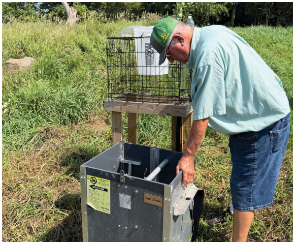
Alan Ottens checks out one of the many tile monitoring systems set up to monitor field-to-stream conditions.
