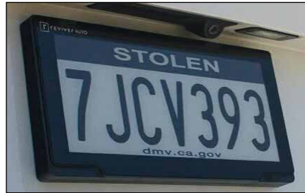
Reviver's digital license plate shows an example of a stolen car, left, and an Amber Alert.
