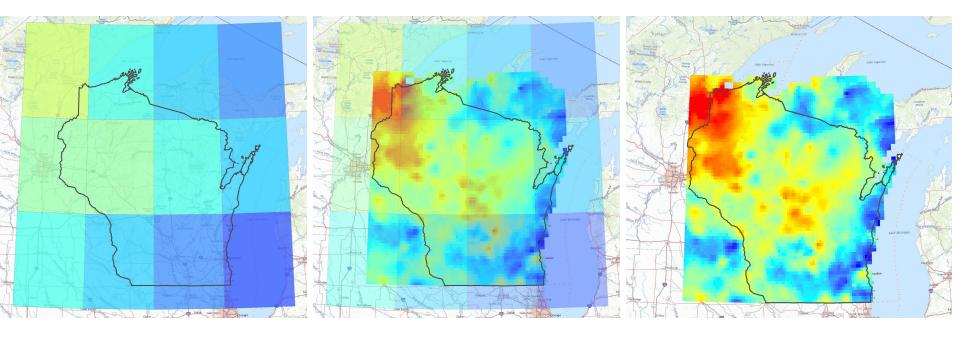
Example of "downscaling" from a global climate model, a general circulation model (GCM), to a regional and more detailed scale to better show and understand high and low temperatures. Sources: Dr. Eric Compas, UW-Whitewater; Lawrence Livermore National Laboratory; USGS
