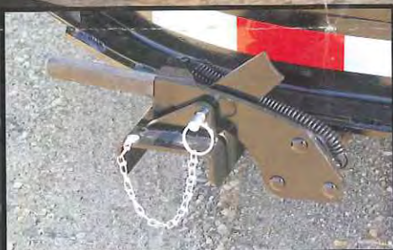
Single-lever, twin-latch system keeps deck secured to the frame.
