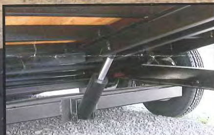
Deck cushion cylinder controls the deck while it closes with equipment loaded.
