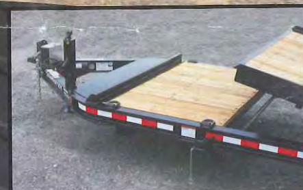
The Stationary Deck option gives you an additional four feet of stationary deck.
