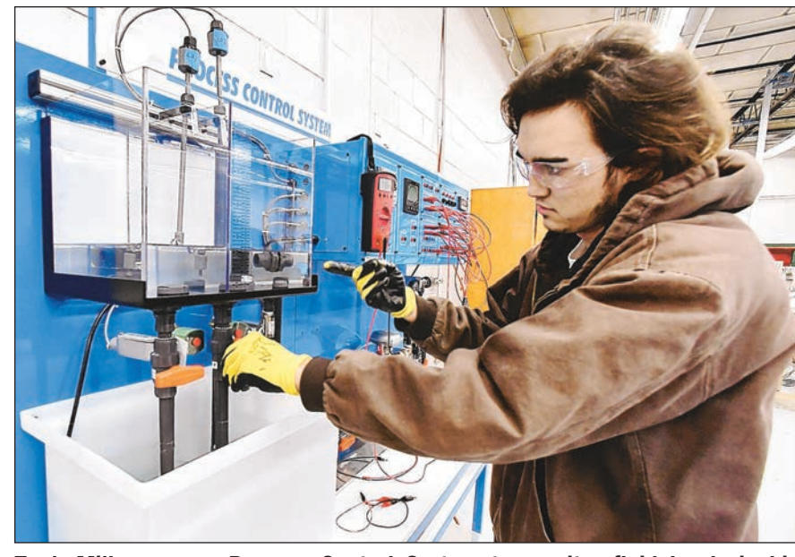
Zach Miller uses a Process Control System to monitor fluid levels in his Withlacoochee Technical College Industrial Machinery and Controls program.
