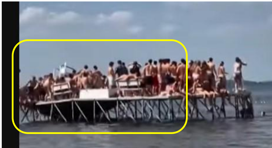
5) Support legs towards the south side are now failing. 1 second elapsed from initial buckling.
