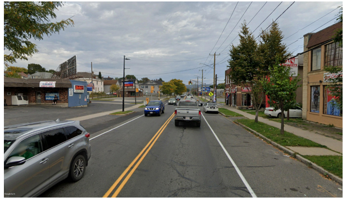
Tyler Street: Example of LTS 3 Source: Google Earth Streetview
