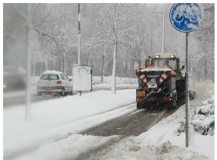
Narrow snow removal machines used to haul away snow from separated bike lanes.
