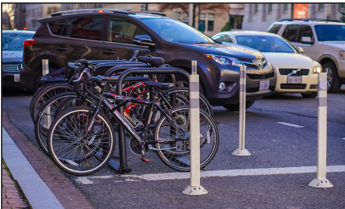
Bicycle parking racks located on a street within on-street car parking width. The bicycle racks are protected with flexposts, or bollards, to improve visibility. Given the proximity to moving vehicles, safety precautions should be taken to ensure people parking their bikes are safe and adequately removed from traffic.
