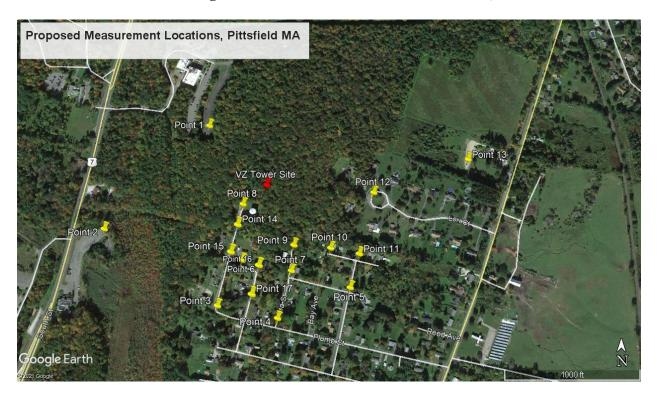
The field measurement results indicate that the maximum level of RF energy emitted from the Pittsfield SE site located at 877 South Street, to which the general public ("general population/uncontrolled") may be exposed to, is below all applicable federal health and safety limits. Specifically, the field measurements show that the maximum level of RF emissions measured near the Pittsfield SE site is **1.66** % of the FCC Standard for the public environment.
