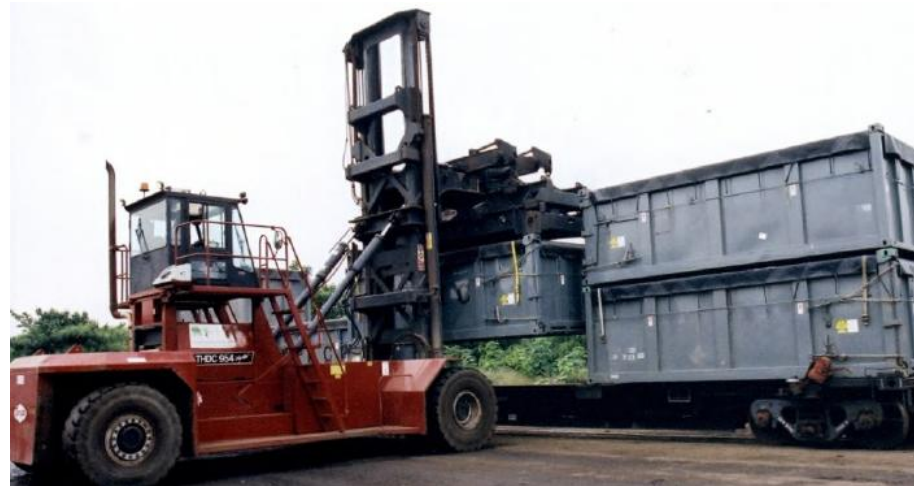
Loading container to rail
