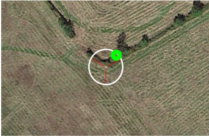
Figure 5. Current conditions and tower/guy line placement at proposed site for October Mountain Motus receiving station off Washington Mountain Road in Washington. Shown are: Steel guy line anchored 23ft from tower base (red lines), tower area (white circle), and an adjacent tree (green mark) depicted in Figures 6 & 7.
