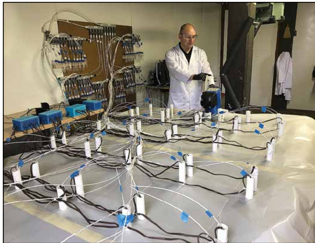
Brian Shedd, a geologist with the Baltimore District of the U.S. Army Corps of Engineers, checks a pump used to control the flow of water through the aquifer mockup set up at a lab in an old guardhouse and ordnance storehouse by Fort McHenry on Baltimore's harbor. The scale model, used to test the flow of contaminants through soil and groundwater, is a shallow tank filled with clean, sandy soil from an Army installation in New York, with a grid of monitoring wells inserted to track and sample liquids as they move through it. (Timothy B. Wheeler)
