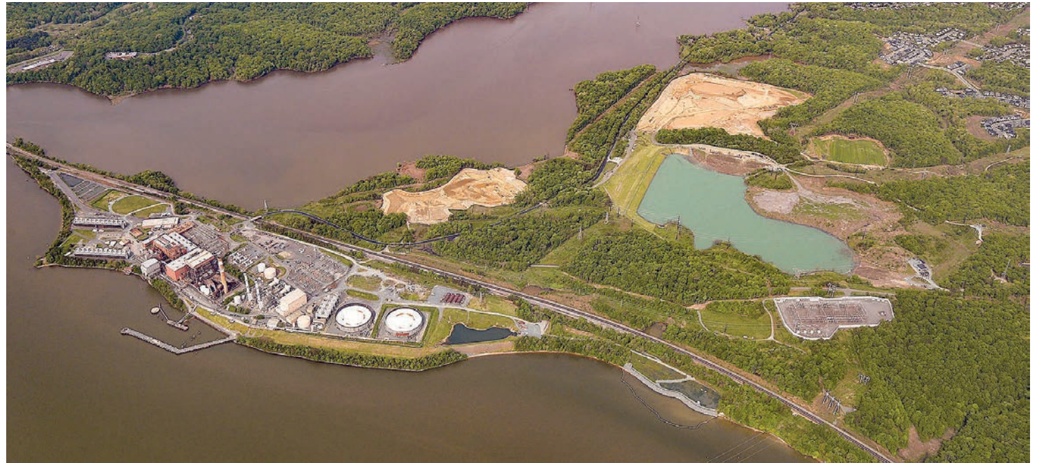
The Possum Point Power Station, near the Virginia shore of the Potomac River at Quantico Creek, burned coal from 1948 to 2002, using expansive ponds to store the coal ash waste. (Courtesy of Dominion Energy)
