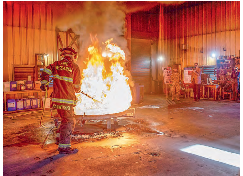
Engineering technician Stanley Karwoski extinguishes a fire during a test at the U.S. Naval Research Laboratory near Chesapeake Beach, MD. The test was part of an effort to compare the firefighting performance of foams that don't contain PFAS and those that do. (U.S. Navy/Jonathan Sunderman)
