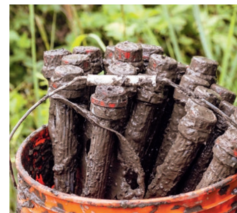
Spears used to extract contaminants from the Anacostia marsh stand in a bucket. (Dave Harp)
