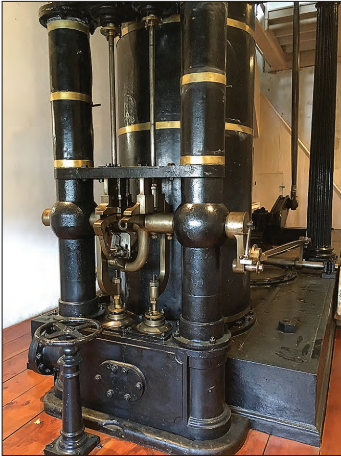
Two engines, one of which is shown here, flanked a large, bucket-bearing wheel that was used to raise the water level in the C&D Canal and lock until 1927.
