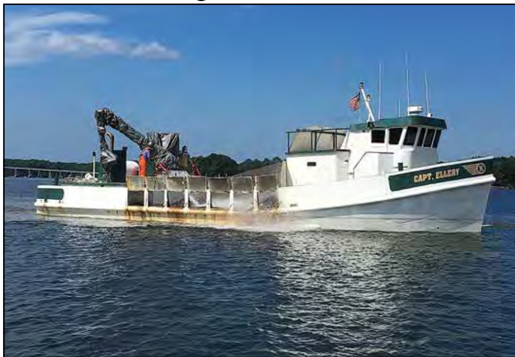
Water cannons aboard the Capt. Ellery, a boat owned by the W. E. Kellum seafood company, spray crushed granite into the Piankatank River. The golf ball-size stones were being placed in a 6- to 8-inch layer over 15 acres of river bottom to provide artificial substrate on which oyster spat may settle and grow. (Timothy B. Wheeler)
