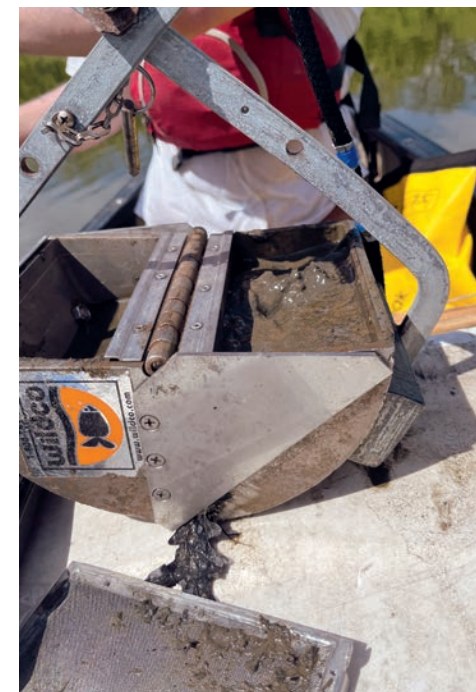
A sampling device holds muck grabbed from the Potomac River bottom during a mid-April monitoring paddle organized by the Potomac Riverkeeper Network. (Courtesy of Potomac Riverkeeper Network)
