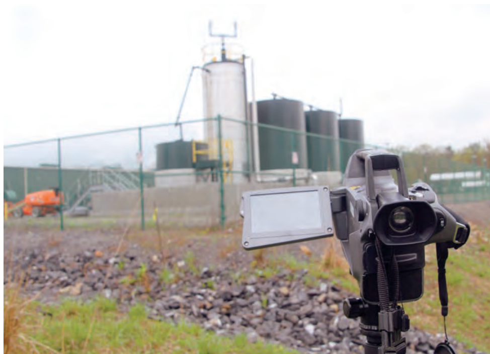
This infrared camera was used to capture images of methane escaping a natural gas well in Lycoming County, PA. (Earthworks)
