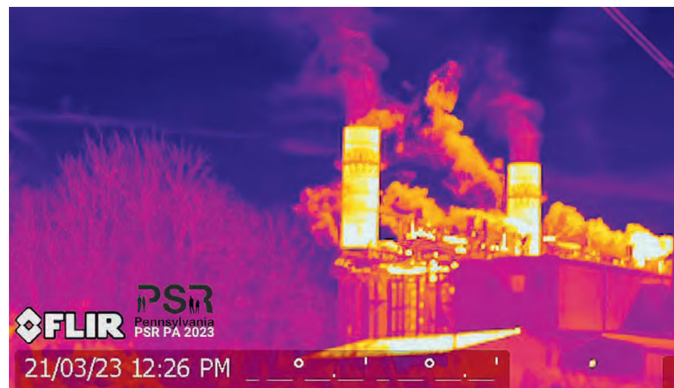
A camera that sees infrared lightwaves captured this daytime image of methane emissions (the orange “smoke”) from a gas-fired power plant in Pennsylvania. These emissions are not visible to the naked eye. (Physicians for Social Responsibility, PA Chapter)
