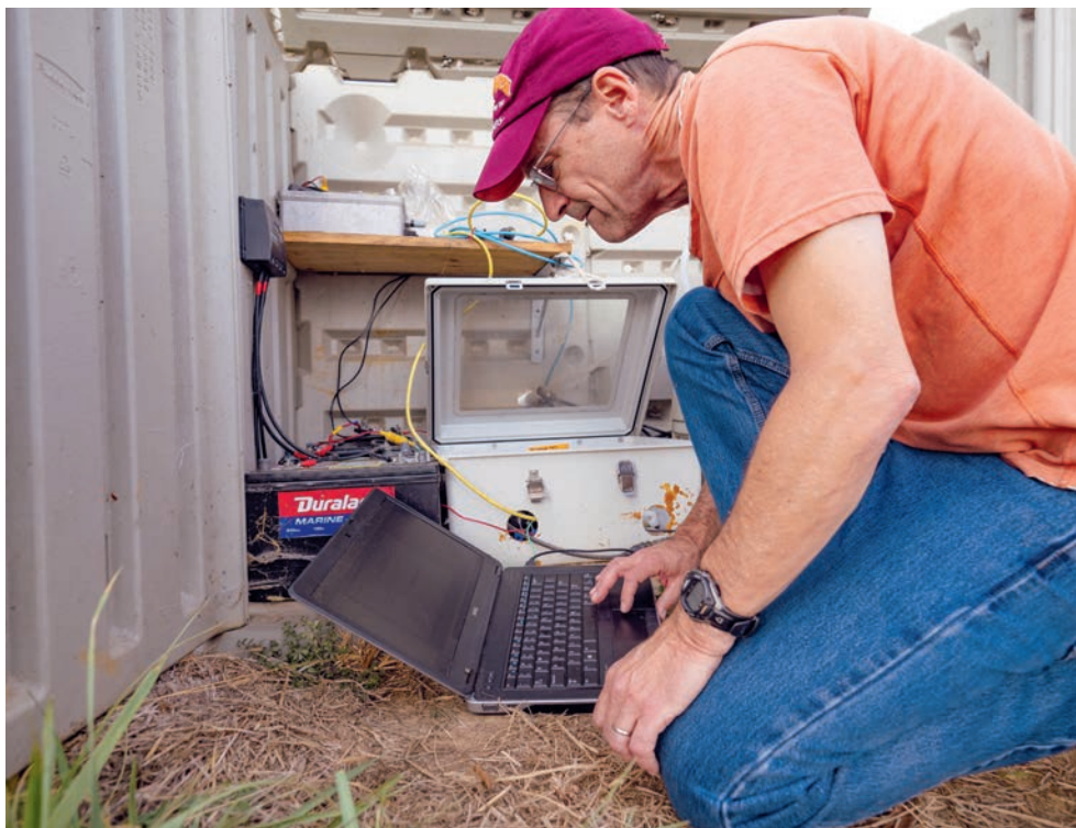
Kurt Stephenson of Virginia Tech examines data collected by instruments that continuously monitor how well a bioreactor in Rockingham County, VA, removes nitrogen from a stream. (Dave Harp)
