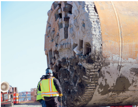
A gigantic tunnel-boring machine, nicknamed Hazel, sees the sun for the first time in 16 months, having completed a 2-mile stormwater tunnel in Alexandria, VA. (AlexRenew)
