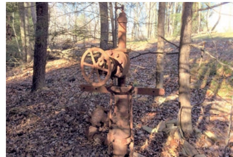
This abandoned natural gas well was found to be leaking gas after a nearby garage exploded in western Pennsylvania. (Pennsylvania Department of Environmental Protection)
