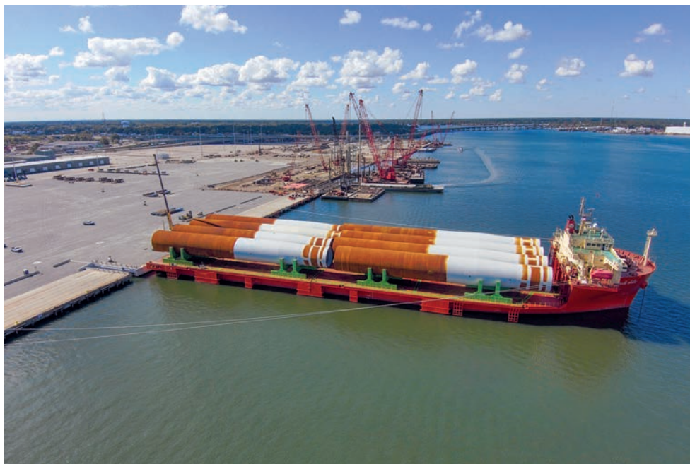
A specialized ship at the Portsmouth Marine Terminal in Virginia is loaded with sections of "monopile" that will support the wind turbines being built offshore. (Courtesy of Dominion Energy)
