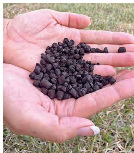
These carbon-rich pellets, or biochar, were made by burning leaf waste. (U.S. Department of Agriculture)
