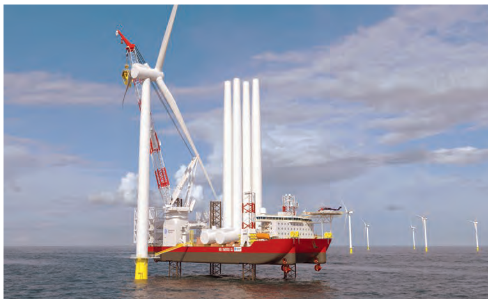
This rendering illustrates the vessel that will transport and install the foundations and turbines for a wind facility offshore of Virginia. (Courtesy of Dominion Energy)
