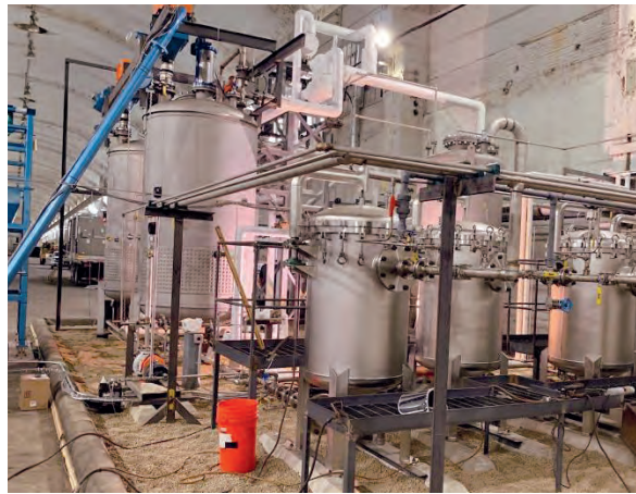
This Pennsylvania facility successfully extracted valuable elements from ash waste left over by coal-fired power production. (Winner Water Services)
