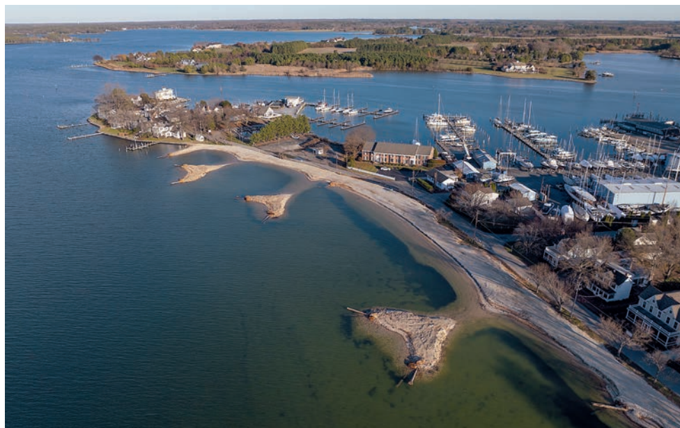
The town of Oxford, MD, is constructing a living shoreline to restore and protect a stretch of land known as the Strand. The area will be planted with native vegetation later this year. (Dave Harp)
