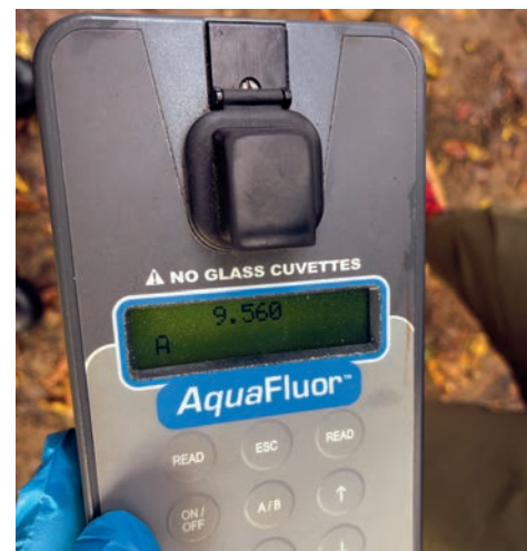
Blue Water Baltimore uses this device to test for the presence of wastewater in streams. (Timothy B. Wheeler)
