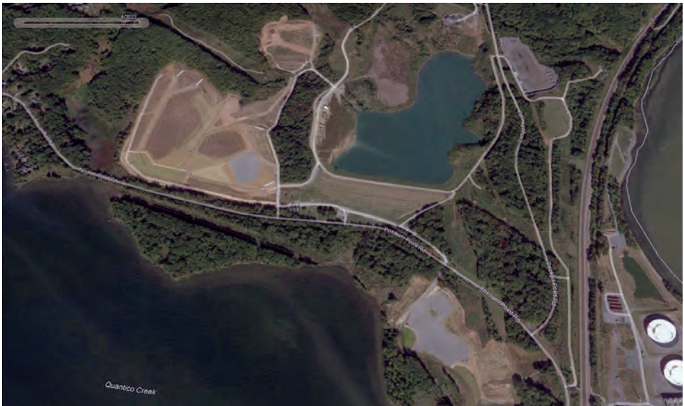
Two former coal ash storage pits are marked by brown and gray patches at Dominion’s Possum Point Power Station along the Potomac River in Virginia. The ash has been moved to a storage pond, visible in the center, while the company seeks approval for a new onsite landfill. (Dominion Energy)
