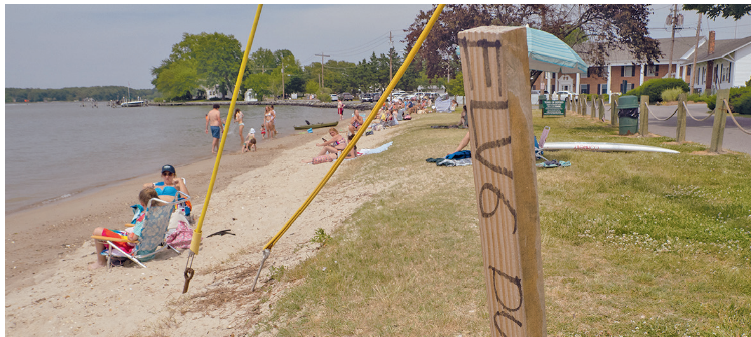
A wooden stake marks where a dune will be constructed to help protect the swimming beach and nearby road along the Tred Avon River in Oxford, MD. Vegetated islands are to be installed just offshore to buffer the shoreline from wave erosion. (Dave Harp)
