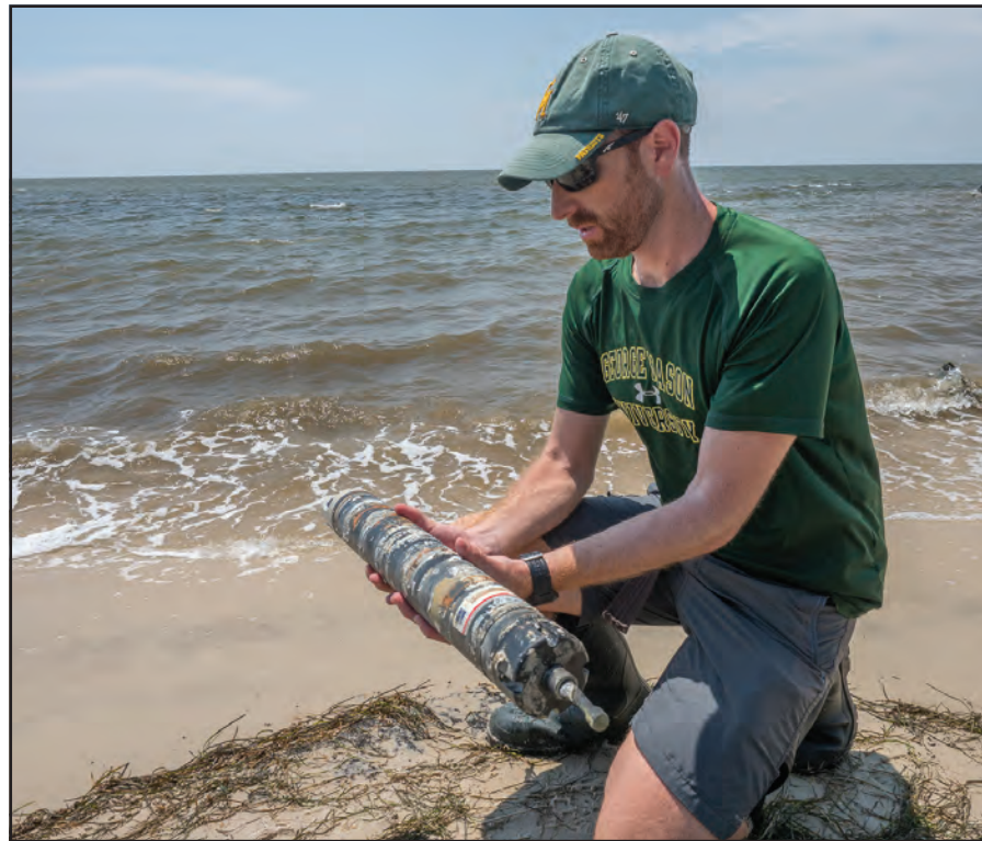
Juan Garzon, a doctoral student in coastal engineering at George Mason University, holds an acoustic Doppler current profiler, which is deployed in the shallows to measure currents or water velocity from the bottom to the surface. (Dave Harp)
