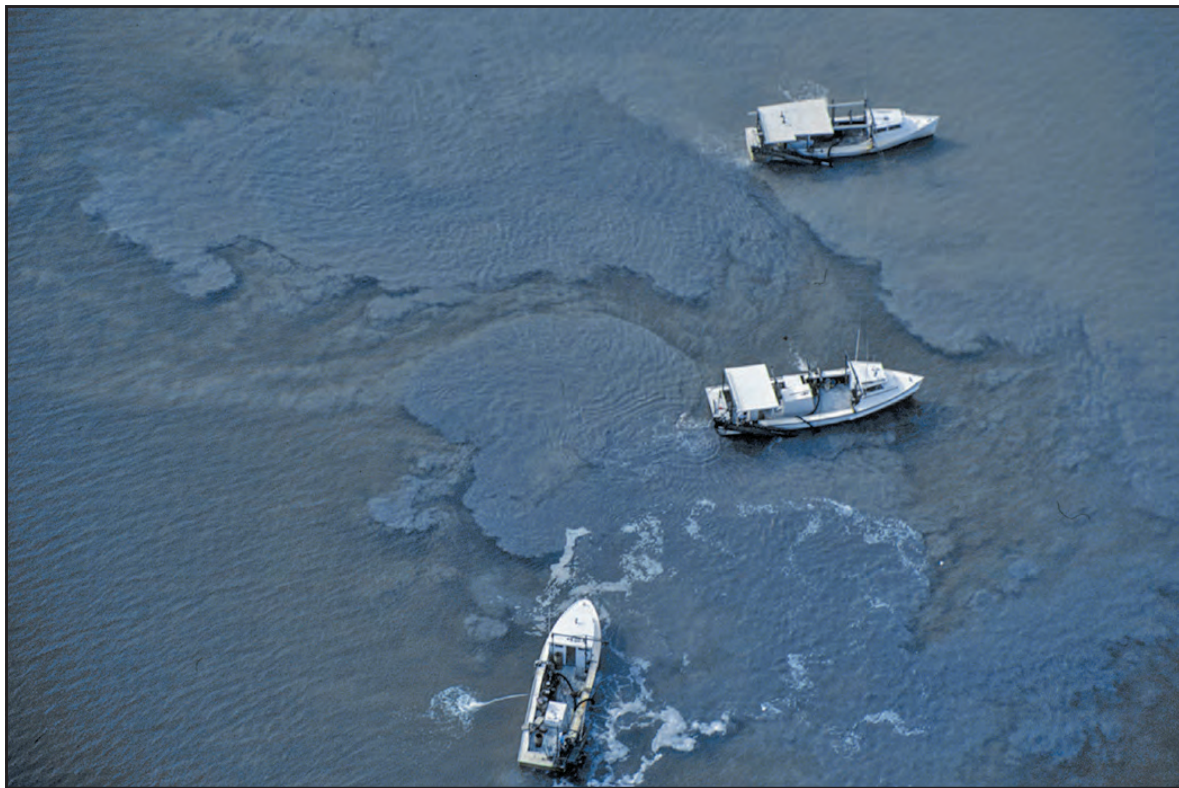
During hydraulic dredging, a suction tube vacuums sediment onto a conveyer belt from which watermen pick out the clams and release the rest back to the water. The process disturbs the bottom and can generate a sediment plume, both of which have the potential to harm the underwater grasses that are often located nearby. (Tyler Campbell)
