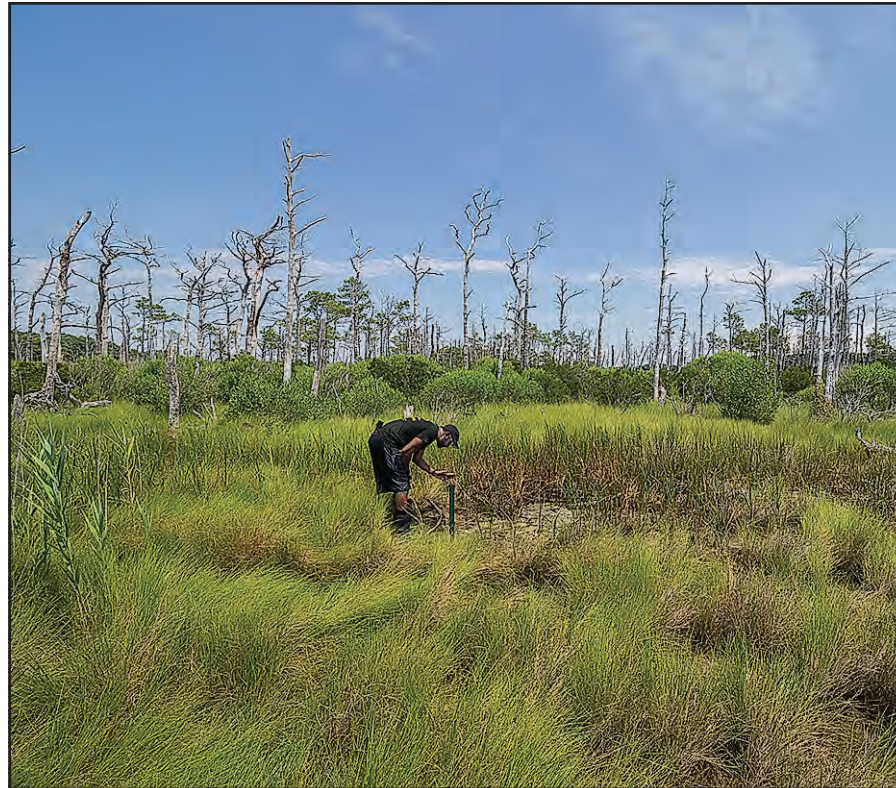
Ali Rezaie, doctoral researcher at George Mason University, checks on a water-level sensor staked out in the marsh back from the beach. Dead trees in the background show the effects of the inland encroachment of brackish water from the Bay. (Dave Harp)
