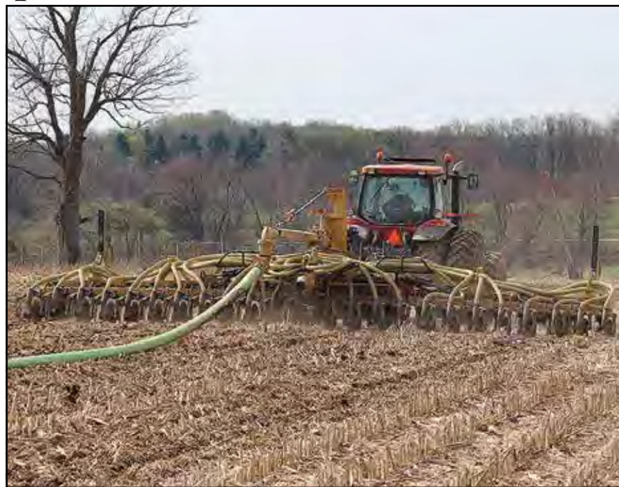
A tractor with an injector fitted with a pipe to pump liquid manure from the farm’s storage facility injects that manure below the surface on a farm in southcentral Pennsylvania. (Penn State Extension)
