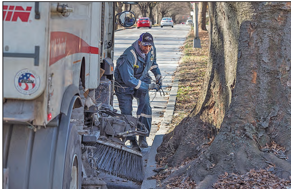
Baltimore city relies heavily on vacuum-powered street sweepers, like the one shown here with its operator Alonzo Ames, to pick up dirt, litter, sediment and other pollutants. Experts' reviews found the practice only modestly effective at cleaning up stormwater, even if done frequently. (Dave Harp)
