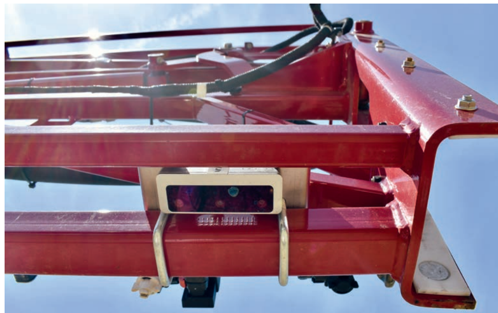
A camera mounted to farming equipment in Beltsville, MD, records plant diversity as it passes over cover crops in April 2025. (Matt Kane/The Nature Conservancy)
