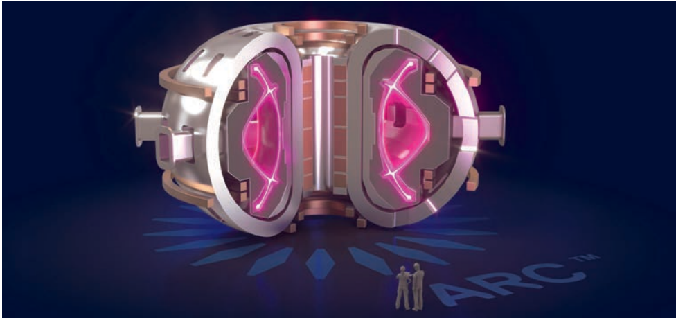
Commonwealth Fusion Systems aims to generate energy from a nuclear fusion process using a tokamak, a donut-shaped container comprised of electromagnets that confine, shape and drive plasma. (Commonwealth Fusion Systems)
