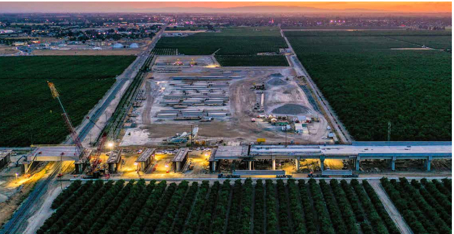
The Hanford Viaduct spans 6,333-feet long and will take high-speed trains over the highway or to the Kings/Tulare Regional Station.
