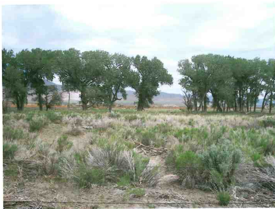
Picture 21 At Section 8 looking toward NE.-Left overbank Manning's n=0.05
