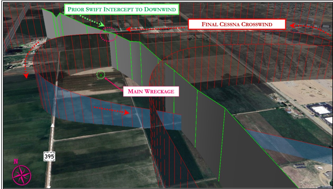
Figure 05: Comparison of the Cessna's accident flight track and the Swift pilot's prior flight.
