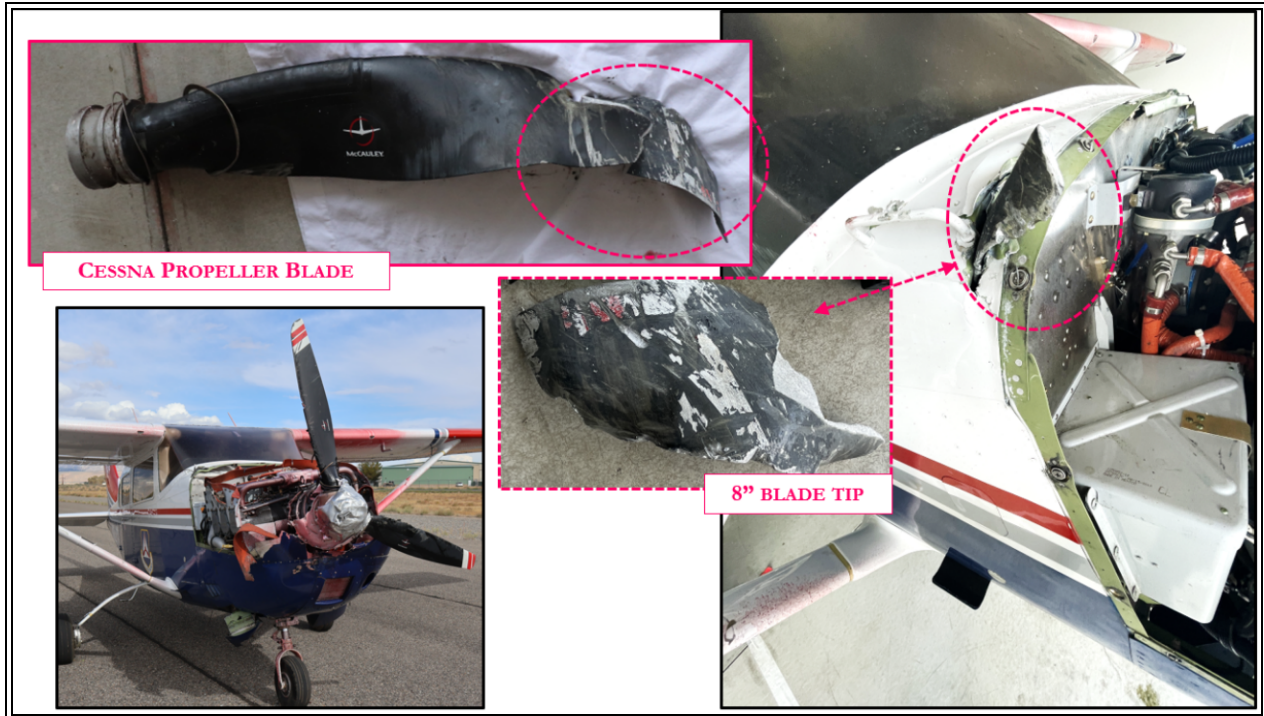
Figure 07: Cessna propeller (missing blade).
